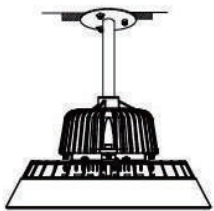
3. Boom installation method
