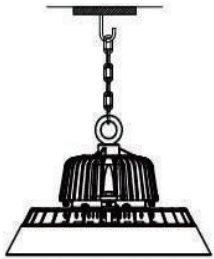
2. Hanging chain installation method
